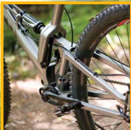
> The Sonix VL120 houses the bottom bracket in the rear triangle attached to the front triangle via a pair of short links.
