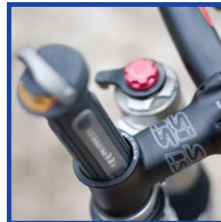
> The one-piece stem acts as the fork steer tube and saves around 150g over the two-piece set up. Cannondale multi tool is an optional extra.
