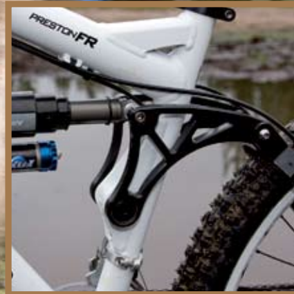
THICK 15MM ROCKER PLATES HELP KEEP THE REAR END FLEX-FREE.
